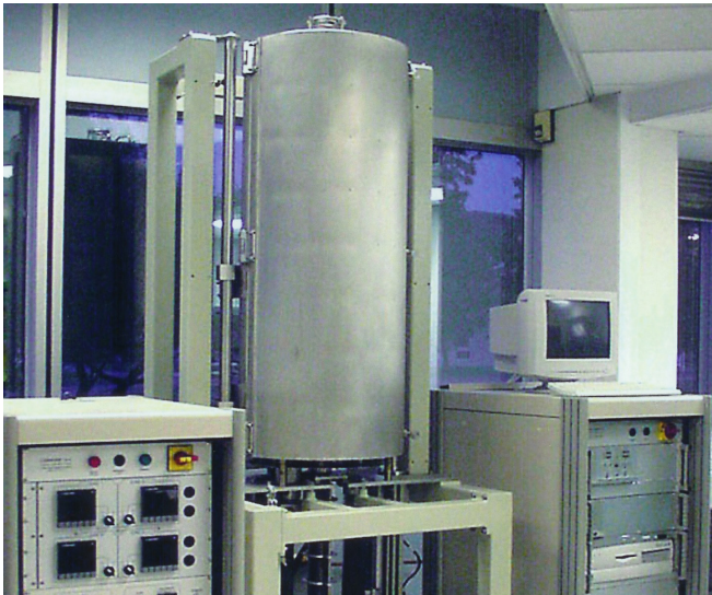
Industrial four zones Bridgman vertical furnace (II - VI compounds) Useful internal diameter: 80 mm Ampoule total travelling length: 600 mm Maximum temperature: 1300°C Maximum gradient in the adiabatic zone: 10°C/cm
