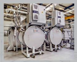
**FLEX modular** Oil quenching (hot or cold), HPGQ, reversible (up to 20 bar) and heating cells, flexible for multiple processes and max. capacity. Adaptable for total automation.
