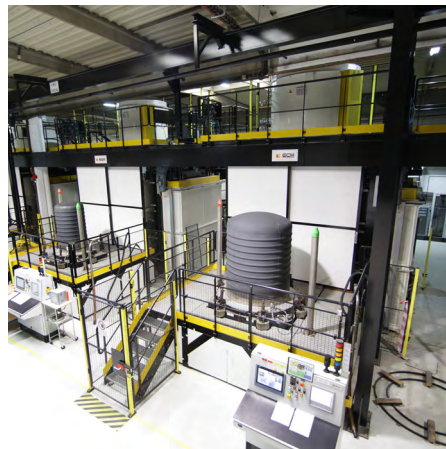
Vapor Phase Aluminization (VPA), VPC and FIC furnaces for protective coatings against high temperature oxidation and hot corrosion. AMS Compliant. Diameters from 700mm to 1500mm.
