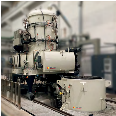
The PFTH furnace consists of a heating cell and pit oil quenching cell. It is a fully automated installation, guaranteeing high reproducibility.
